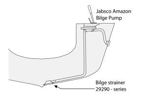
These are the traditional mainstay of small craft bilge pumping systems and can offer surprisingly good flow rates, as well as a variety of installation options. Yacht racing rules state that at least one pump must be capable of being pumped from the cockpit with all hatches shut. The best way to accomplish this is with a through deck kit which allows the pump to be in stalled safely below decks while the operator pumps from above.
