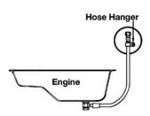
The Jabsco Oil Drain Hose includes a drain plug fitting, oil drain hose assembly, hose hanger and a cap. This provides an easy method of connecting to several pump types for neat and easy oil removal.
