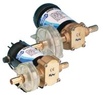
These robust pumps make oil and diesel transfer simple and easy for fixed installation systems. The Junior Gear Puppy can produce 3.5 gpm (14 lpm) and the Gear Puppy can produce up to 6.5 gpm (25 lpm) and handle viscosities up to 150cs.
